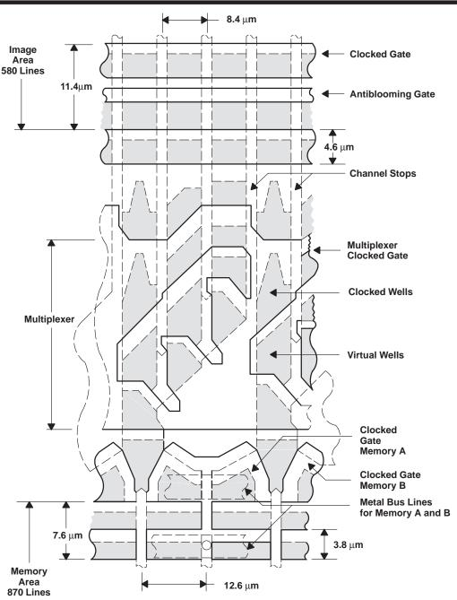
Figure 1. Layout of Multiplexing Gate
