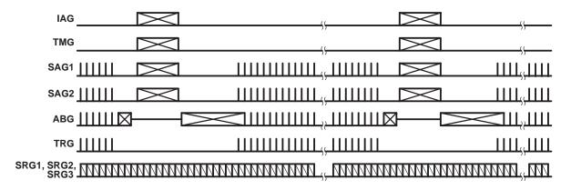
Figure 7. Vertical Timing, Low-Light Mode
