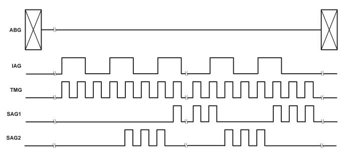
Figure 10. Parallel-Transfer Timing
