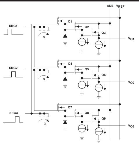
Figure 3. Circuit Diagram – Charge-Detection Amplifiers
