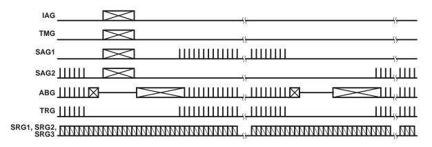
Figure 8. Vertical Timing, Still Mode
