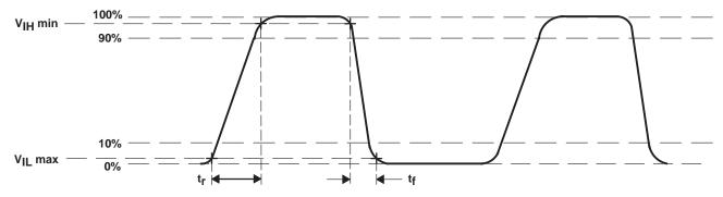
Slew rate between 10% and 90% = 300 V/µs,  $t_{f}$  =  $t_{f}$  = 15 ns
