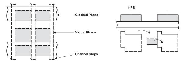
Figure 5. Charge-Transfer Process
