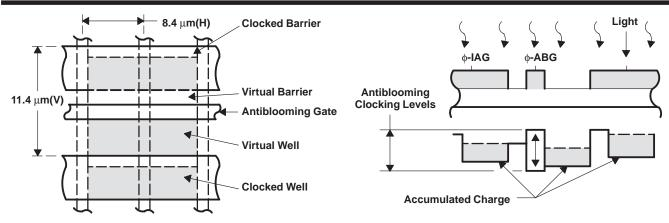
Figure 4. Charge-Accumulation Process
