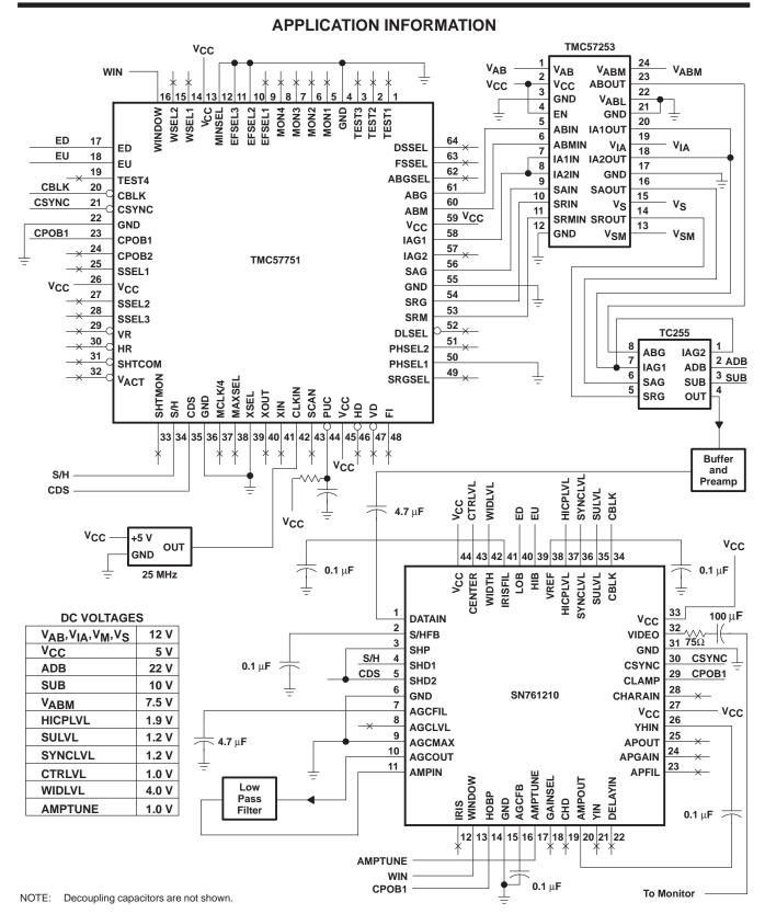
Figure 13. Typical Application Circuit
