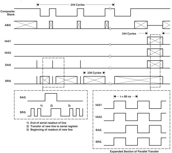
Figure 3. Timing Diagram
