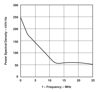
Figure 12. Noise Power Spectral Density
