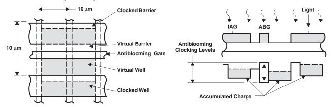
Figure 1. Charge-Accumulation Process
