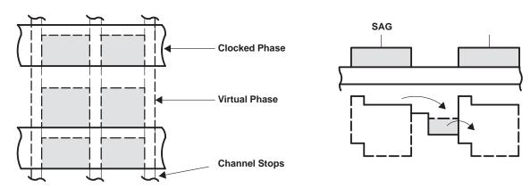
Figure 2. Charge-Transfer Process
