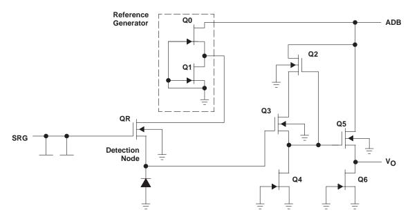
Figure 4. Output Amplifier and Charge-Detection Node
