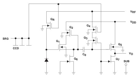
Figure 4. Charge-Detection Schematic
