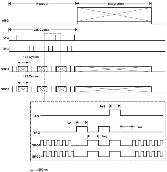
$\begin{array}{l} t_{W1} \geq 600 \text{ ns} \\ t_{W2} \geq 600 \text{ ns} \\ t_{W3} \geq 600 \text{ ns} \\ t_{W4} \geq 125 \text{ ns} \end{array}$
