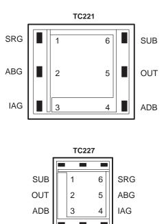
The TC221 and TC227 are supplied in 6-pin molded plastic packages; the TC225 is supplied in a 10-pin molded plastic package. The glass window can be cleaned using any standard method for cleaning optical assemblies or by wiping the surface with a cotton swab soaked in alcohol.
